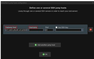
In the second step, the tab **Network settings** must be selected. There you have to click on **SSH gateway (jump host)** to specify the SSH host. Don't be surprised there are no changes shown in this window, after the next step.
