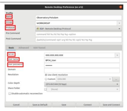
If access is not via the local IP address space, an SSH tunnel must be established. To do this, you should select the SSH Tunnel tab in the profile configuration-window (see image below). After that you have to select Custom, set the server name to one of the computers of the Astro Cluster, e.g. prakt.astro.physk.uni-potsdam.de and use a valid user name like castor. If authentication is not done by public key cryptography, the Password must be set as well.
