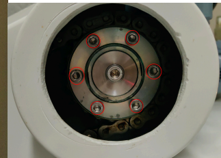
Fig. 4: Slipping clutch with Allen screws
