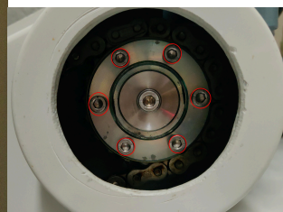
Fig. 4: Slipping clutch with Allen screws
