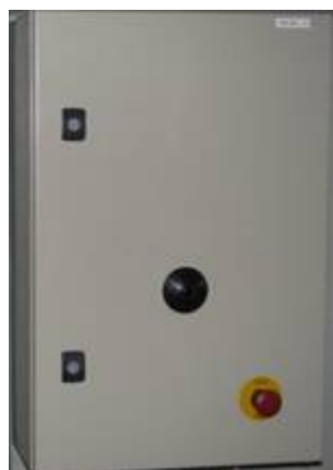
Control box with the emergency button
