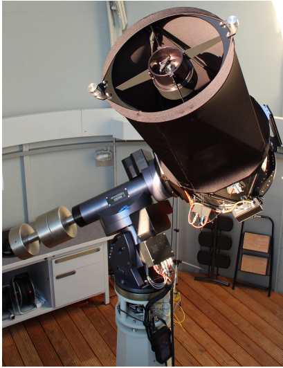
OST 2.0 - Our new Telescope a CDK20 (Planewave)
