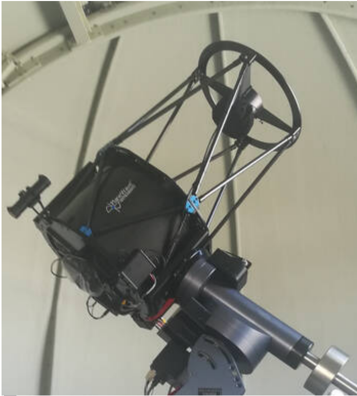
OST 2.0 – Our new Telescope a CDK20 (Planewave)
