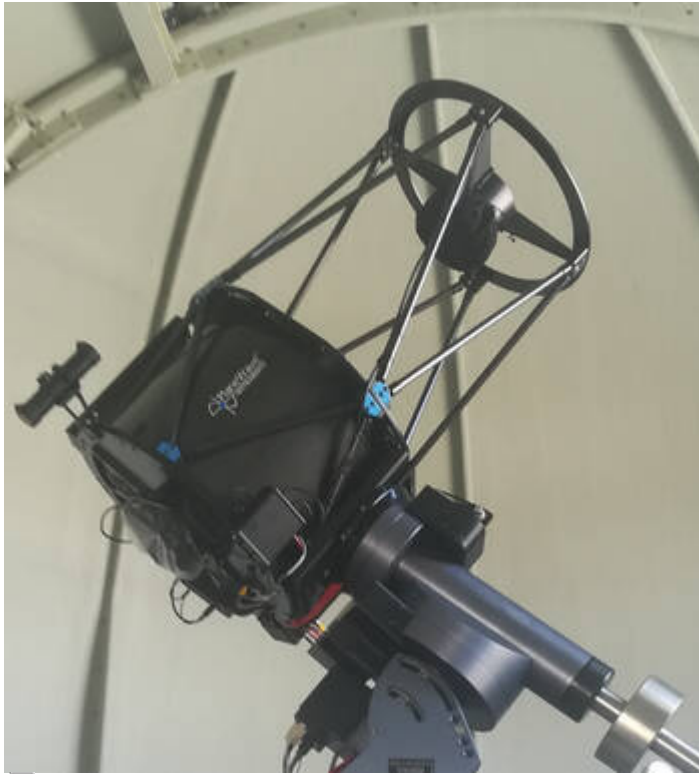
OST 2.0 – Our new Telescope a CDK20 (Planewave)
