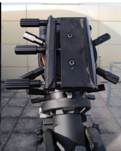
Fig. 14: CGE PRO clamp on the mount
