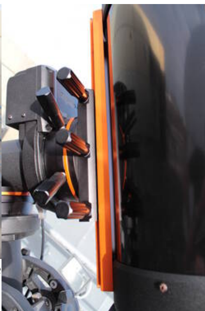
Fig. 15: Attachment of the C11 at the CGE PRO
