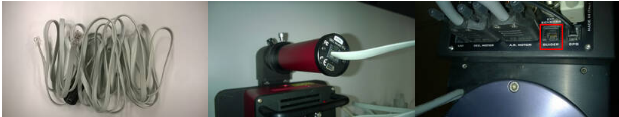
4: Guider cable for the ST-i
