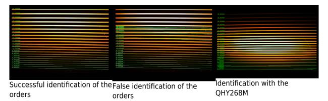
Apart from the number of orders, the width of the orders (Slit order width), and the width of the area within the orders that should be extracted (Slit extraction width) needs to be specified. The default values of 20 pixel are only with restrictions applicable to our combination of BACHES and ST-8. Therefore, these parameters need to be adjusted on a case by case basis.
