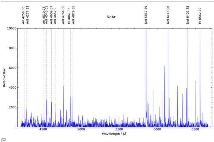
Emission spectrom of our Ne-Ar calibration lamp. The strongest lines are identified.
