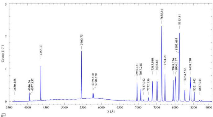
Emission spectrom of our calibration lamp. The strongest mercury and argon lines are identified.
