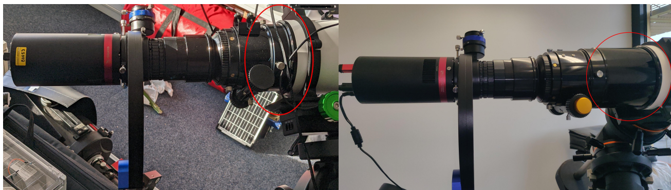
Correct setup without extension tube
