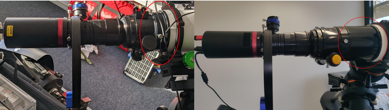
Correct setup without extension tube Incorrect setup with extension tube
