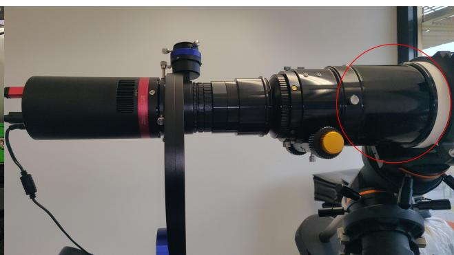
Incorrect setup with extension tube
