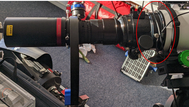
Correct setup without extension tube
