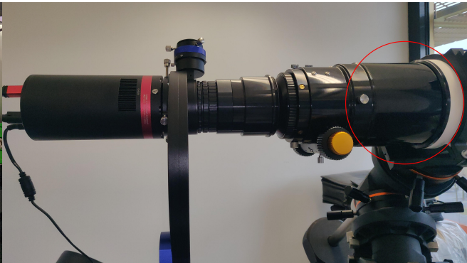
Incorrect setup with extension tube
