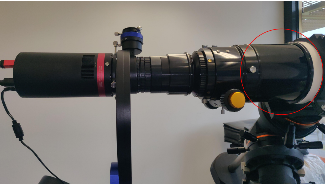
Incorrect setup with extension tube
