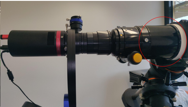
Incorrect setup with extension tube
