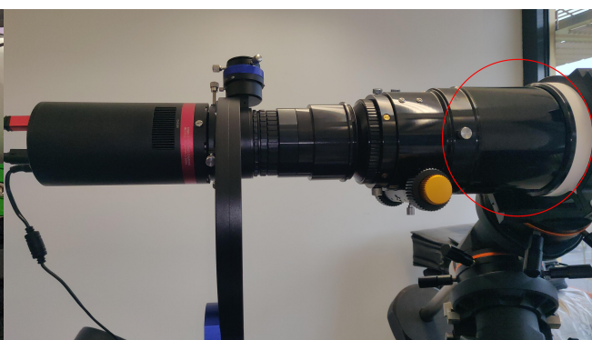
Incorrect setup with extension tube
