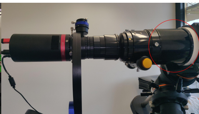
Incorrect setup with extension tube
