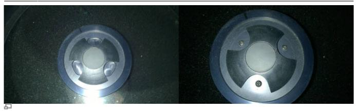
Secondary mirror (right panel: the cover is rotated, so that the screws are visible)
