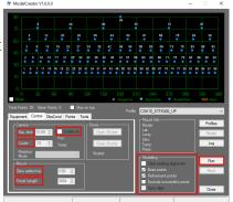
and Sync align are activated. Then *ModelCreator* moves the mount to the first point, takes an image, starts *PlateSolve*, searches for the exact coordinates of the star field, uses this solution to improve the pointing model and continues with the next point.
