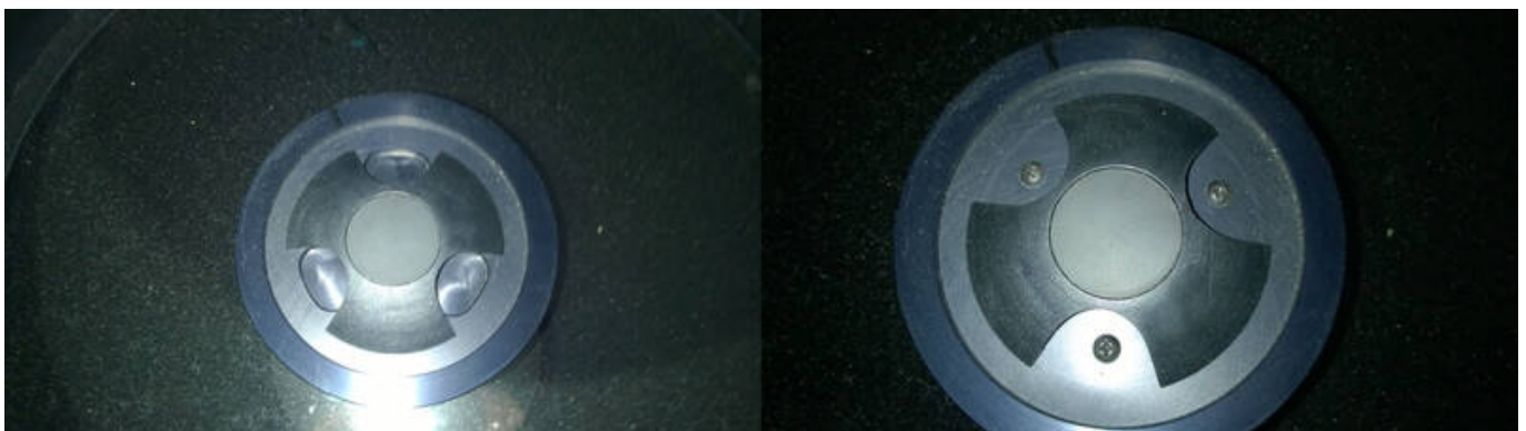
Secondary mirror (right panel: the cover is rotated, so that the screws are visible)
