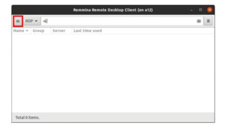
After **Remmina** is started, the first thing to do is to create a new profile by clicking on the button in the upper left corner. The fields Name, Group, Server, Username, and Password need to be set. Name is the name of the profile. Group needs to be set to *WORKGROUP*. Server is the IP of the Observatory Management System (OMS). The Username for everyday use is *BP34\_User*. Password is self-explanatory. Server and Password will be disclosed upon request.
