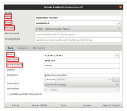
If the access is not from the local IP address space, a SSH tunnel needs to be set up. To do this one has to select the SSH Tunnel tab in the **Remmina** profile configuration window. Afterwards, one needs to select Custom, set the server name to one of the computers of the astro cluster such as *prakt.astro.physik.uni-potsdam.de* and use a valid Username such as *castor*. If the authentication is not by public key cryptography, Password has to be set as well.
