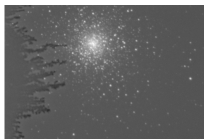
Exposure of the cluster M15 with the ST-8. The left side clearly shows icing on the CCD.
