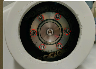
Fig. 4: Slipping clutch with Allen screws
