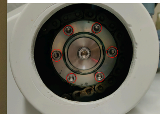
Fig. 4: Slipping clutch with Allen screws
