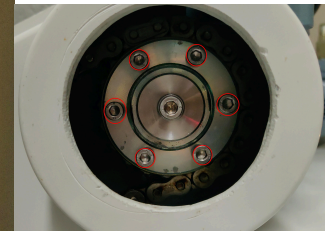
Fig. 4: Slipping clutch with Allen screws
