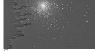
Exposure of the cluster M15 with the ST-8. The left side clearly shows icing on the CCD.
