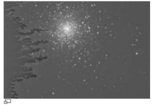
Exposure of the cluster M15 with the ST-8. The left side clearly shows icing on the CCD.
