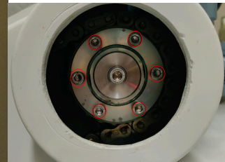
Fig. 4: Slipping clutch with Allen screws
