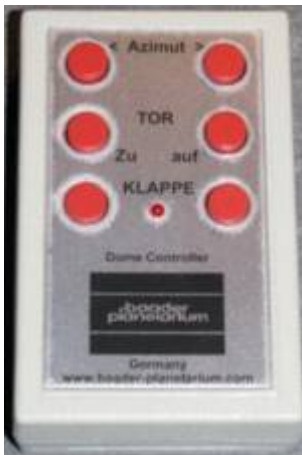
Remote control for the dome
