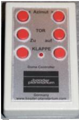
Remote control for the dome
