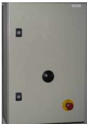
Control box with the emergency button
