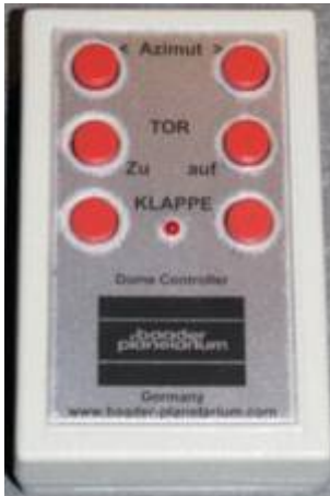
Remote control for the dome
