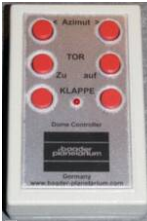
Remote control for the dome
