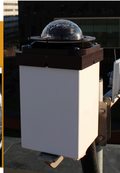
AllSky-340 from SBIG with a little residual moisture from the last rain on the dome
