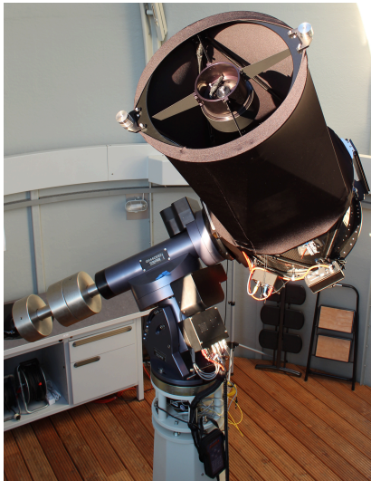
OST 2.0 - Our new Telescope a CDK20 (Planewave)
