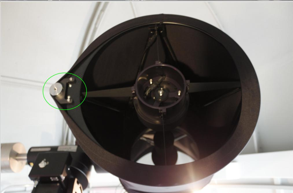
A photograph looking into the front of a telescope tube. The primary mirror is visible in the center. A small, cylindrical counterweight is mounted on the left side of the tube's inner rim. A green circle highlights this counterweight.                                 |
