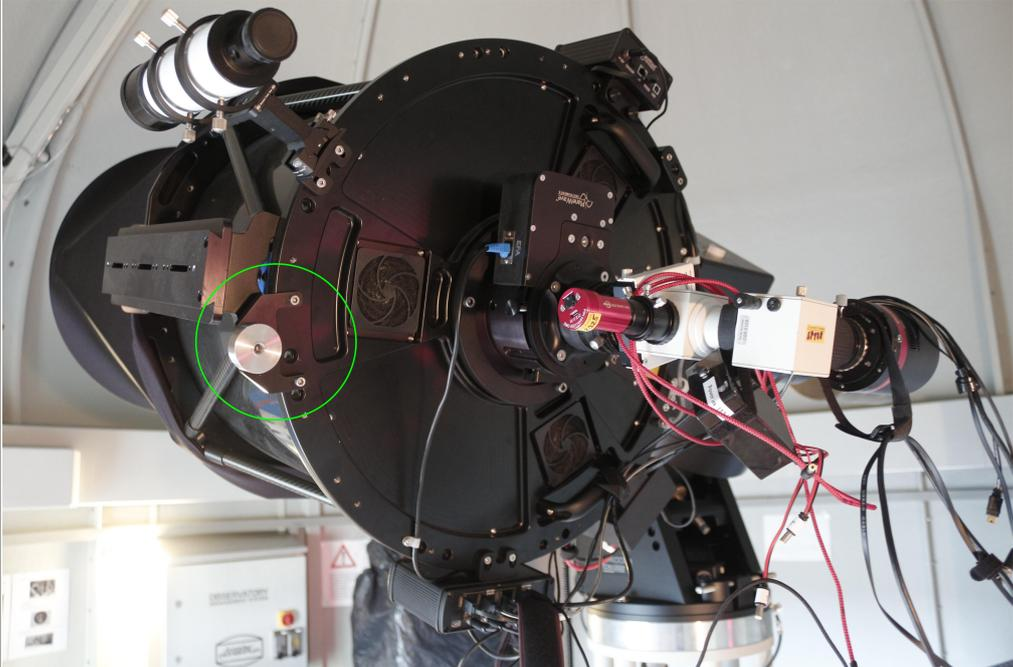
A photograph of a telescope mounted on a tripod inside a dome. The telescope is oriented horizontally. A small, cylindrical counterweight is attached to the back of the telescope tube, highlighted by a green circle. Various cables and electronic components are visible on the right side of the telescope. |
