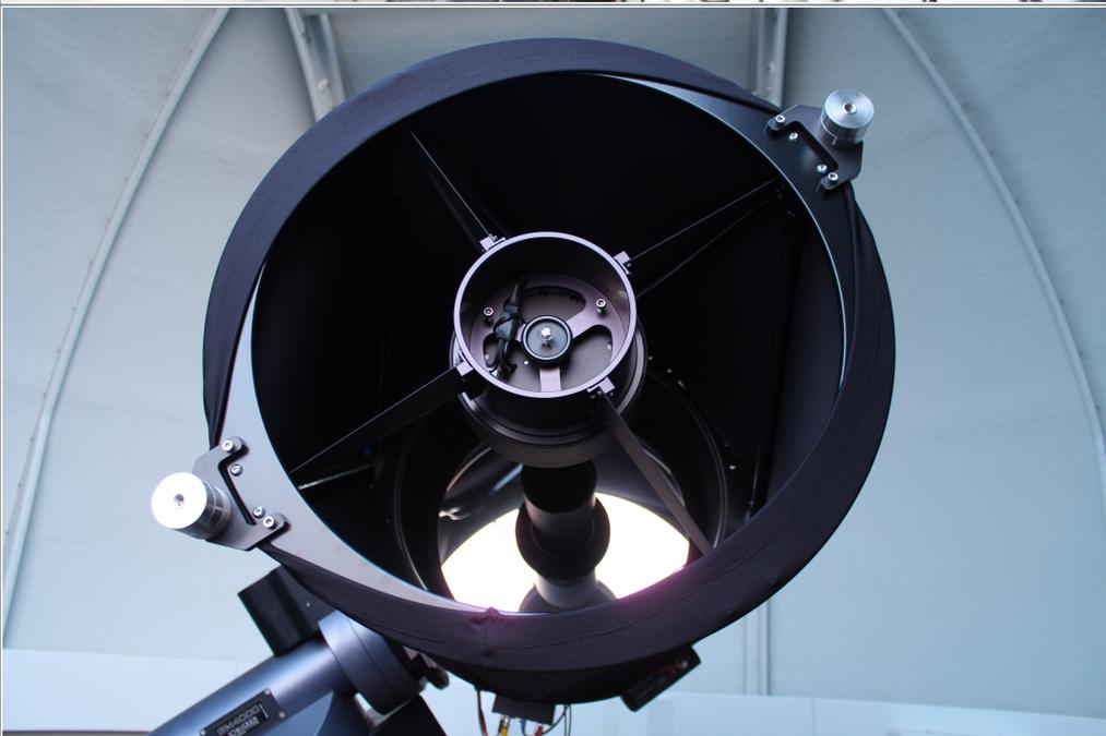
A photograph showing the front view of a telescope. The large primary mirror is visible, and the secondary mirror is mounted in the center. The telescope is mounted on a tripod, and the background shows the interior of a dome.                                                                              |
