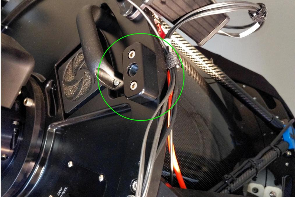
A close-up photograph of the counterweight assembly of a telescope. A black mounting block is attached to a metal bar. The block has two screws and a central hole. A green circle highlights this block. Various cables and mechanical parts are visible in the background. |
