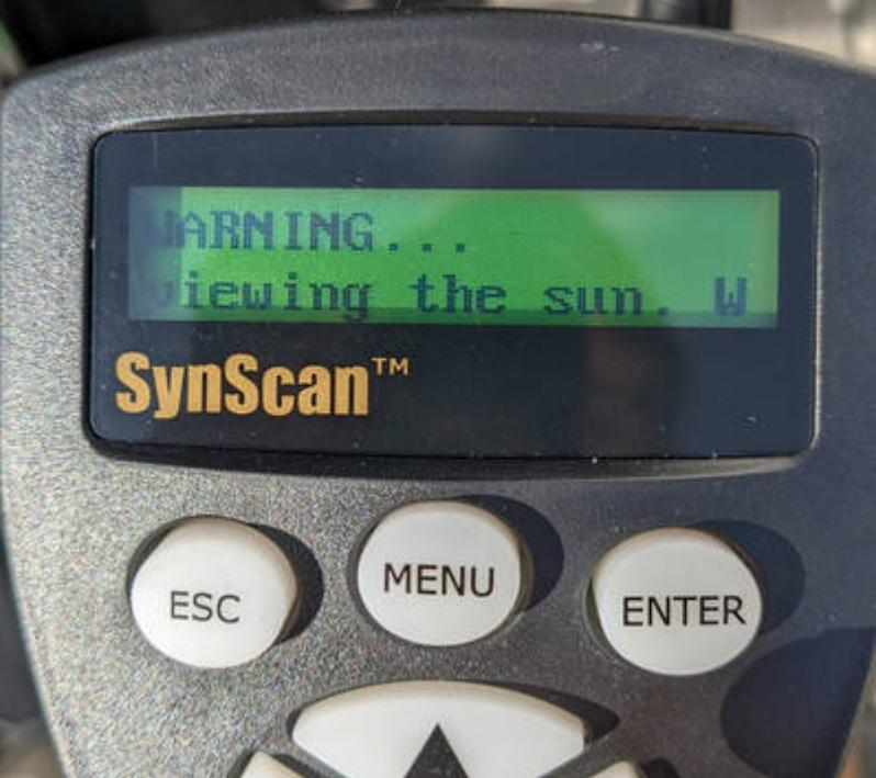
A close-up photograph of a SynScan hand controller. The screen displays a blue-tinted warning message: "WARNING... viewing the sun. W". Below the screen, the "SynScan™" logo is visible. At the bottom of the device, there are three white circular buttons labeled "ESC", "MENU", and "ENTER". A small black arrow pointing upwards is located between the "MENU" and "ENTER" buttons. |
