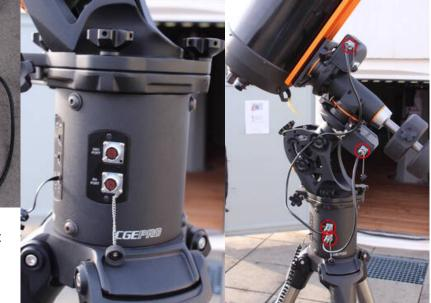
Fig. 8: Electronic box with ports for the cables
