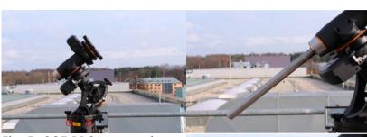
Fig. 5: CGE PRO mounted on the electronic box and the tripod (the red circles indicate two of the bolts that need to be fastened)
