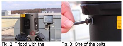
Fig. 2: Tripod with the electronic box (the red circle indicates one of the bolts that needs to be fastened)
