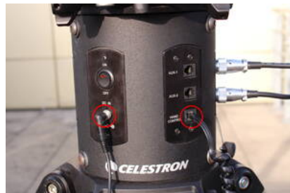
Fig. 12: Ports for the power supply (left) and the hand terminal (right) at the electronic box
