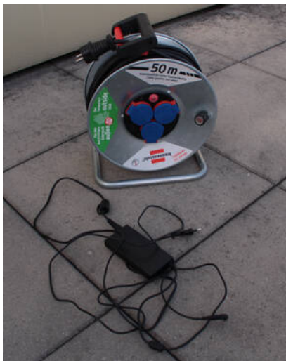
Fig. 10: Mobile power supply and the cable reel
