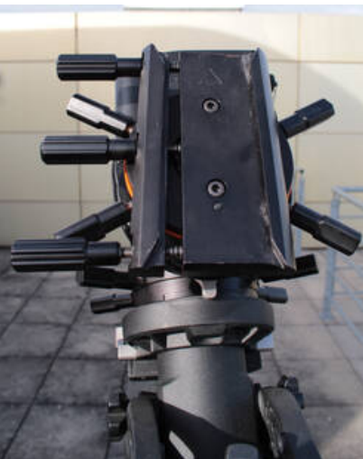
Fig. 14: CGE PRO clamp on the mount
