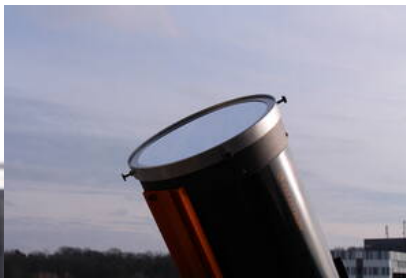
Fig. 17: Tube with the sun filter
