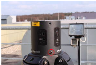
Fig. 2: Tripod with the electronic box (the red circle indicates one of the bolts that needs to be fastened)
