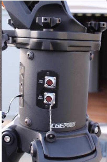
Fig. 8: Electronic box with ports for the cables
