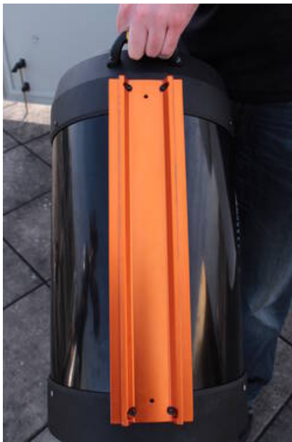
Fig. 13: Dove tail on the tube
