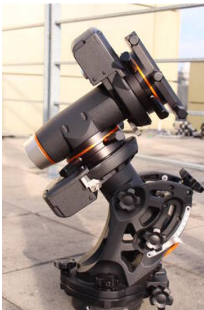
Fig. 5: CGE PRO mounted on the electronic box and the tripod (the red circles indicate two of the bolts that need to be fastened)
