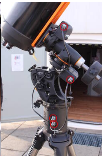
Fig. 9: CGE PRO with the cable attached
