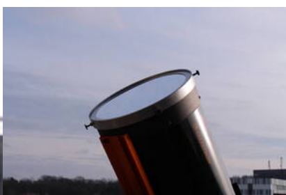
Fig. 17: Tube with the sun filter
