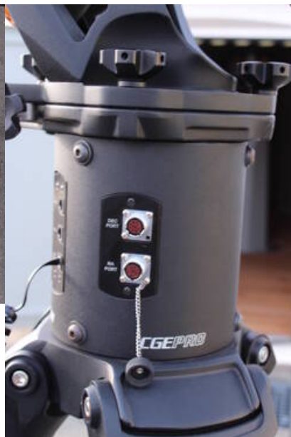
Fig. 8: Electronic box with ports for the cables
