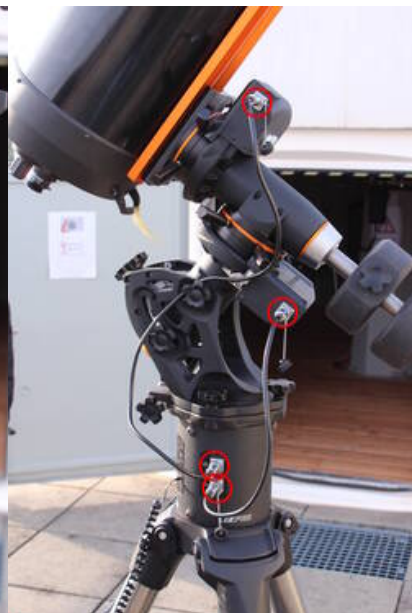
Fig. 9: CGE PRO with the cable attached
