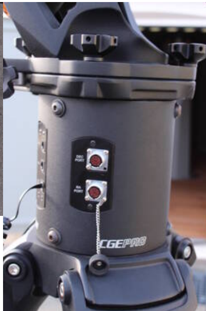
Fig. 8: Electronic box with ports for the cables
