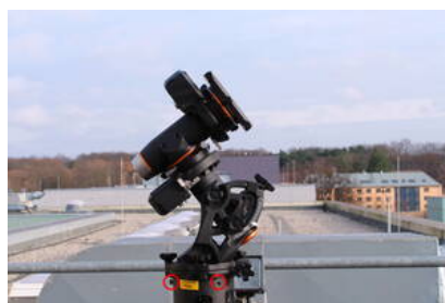
Fig. 5: CGE PRO mounted on the electronic box and the tripod (the red circles indicate two of the bolts that need to be fastened)
