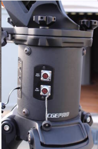
Abb. 8: Electronic box with ports for the cables
