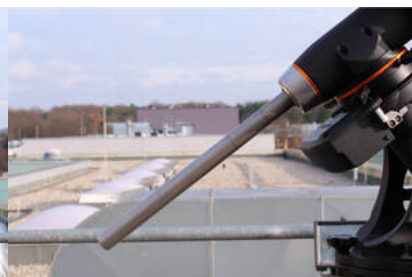
Fig. 6: CGE PRO with the counterweights on the bar
