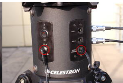
Abb. 12: Ports for the power supply (left) and the hand terminal (right) at the electronic box
