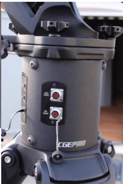
Fig. 8: Electronic box with ports for the cables
