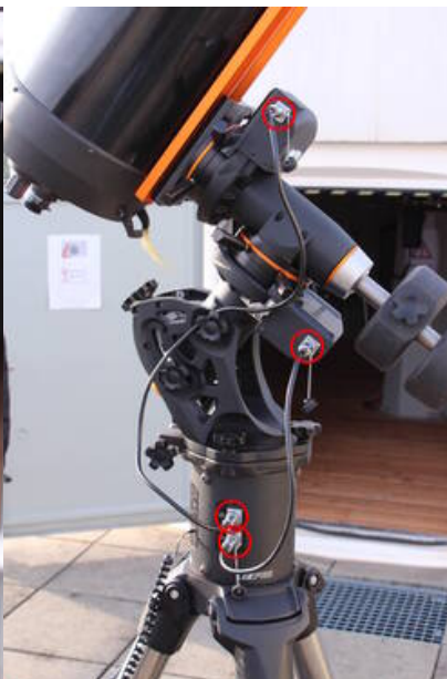
Fig. 9: CGE PRO with the cable attached
