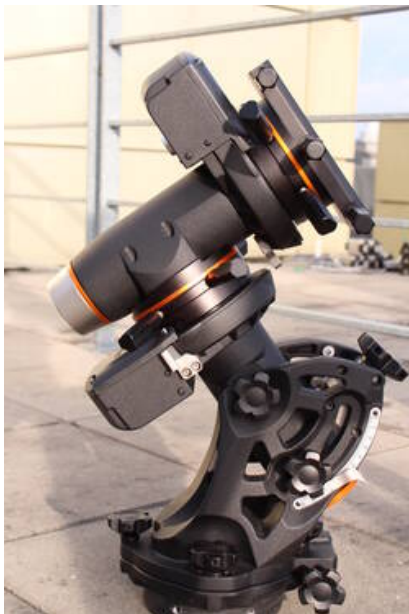
Abb. 5: CGE PRO mounted on the electronic box and the tripod (the red circles indicate two of the bolts that need to be fastened)
