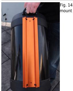
Fig. 13: Dove tail on the tube
