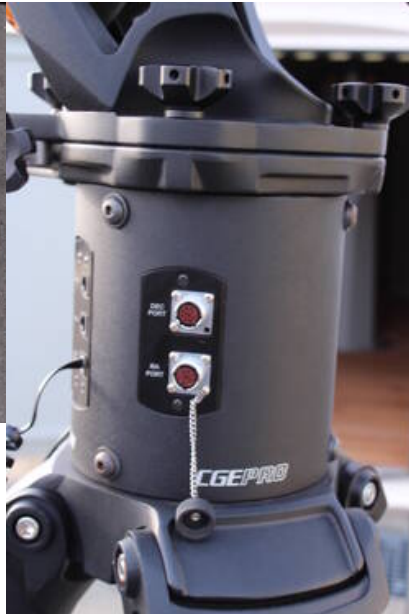
Fig. 8: Electronic box with ports for the cables
