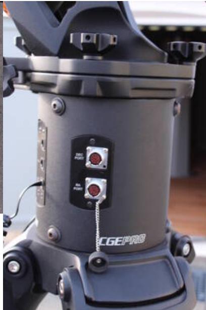
Fig. 8: Electronic box with ports for the cables
