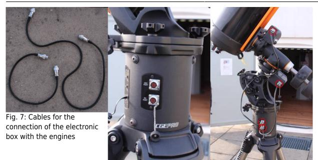
Fig. 8: Electronic box with ports for the cables
