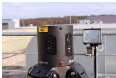
Abb. 2: Tripod with the electronic box (the red circle indicates one of the bolts that needs to be fastened)
