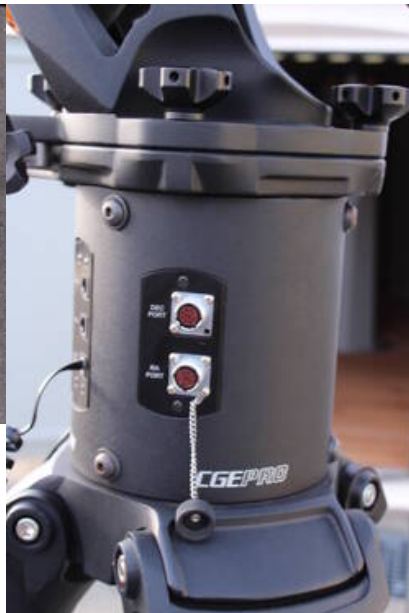
Fig. 8: Electronic box with ports for the cables
