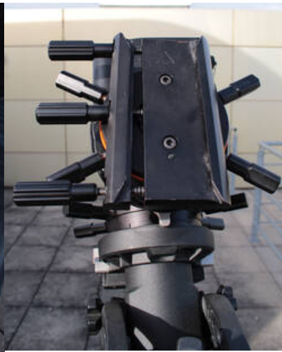
Abb. 14: CGE PRO clamp on the mount
