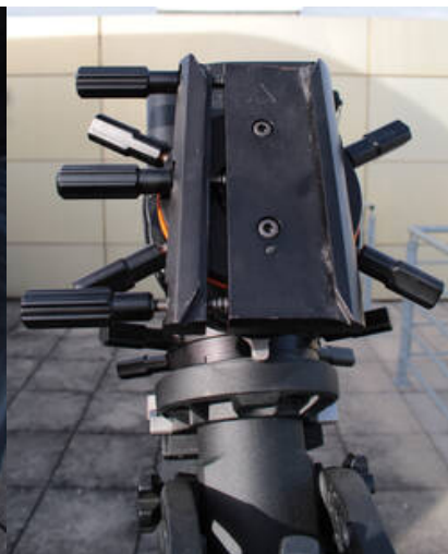
Fig. 14: CGE PRO clamp on the mount
