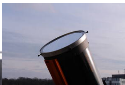
Abb. 17: Tube with the sun filter
