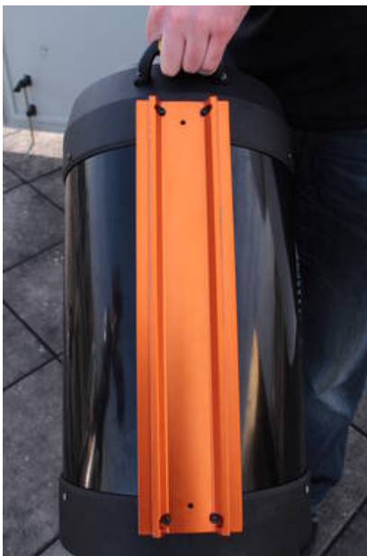
Fig. 13: Dove tail on the tube
