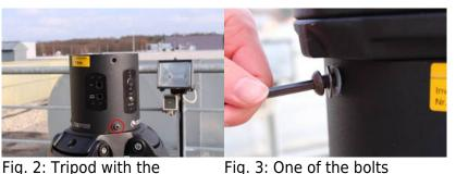
Fig. 2: Tripod with the electronic box (the red circle indicates one of the bolts that needs to be fastened)
