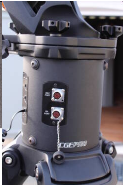
Fig. 8: Electronic box with ports for the cables
