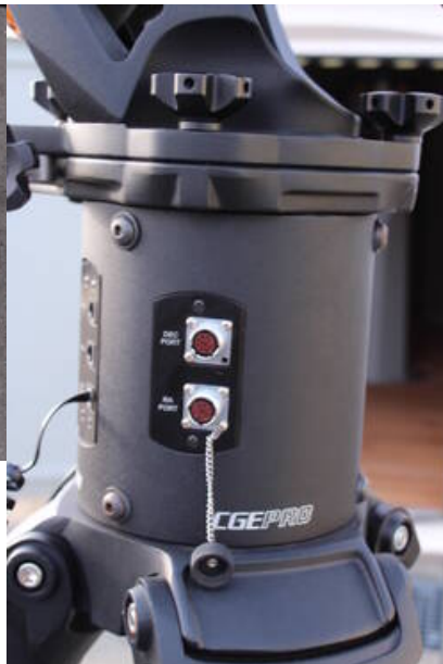
Fig. 8: Electronic box with ports for the cables
