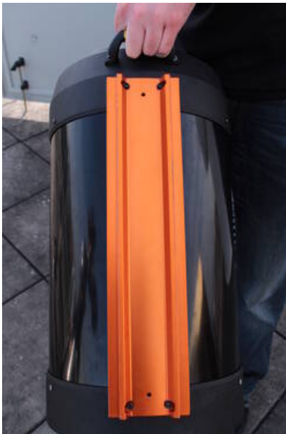
Fig. 13: Dove tail on the tube
