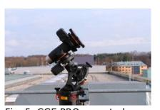
Fig. 5: CGE PRO mounted on the electronic box and the tripod (the red circles indicate two of the bolts that need to be fastened)
