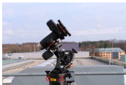
Fig. 5: CGE PRO mounting on electronic box and tripod (the red circles indicate the three bolts to be fastened)
