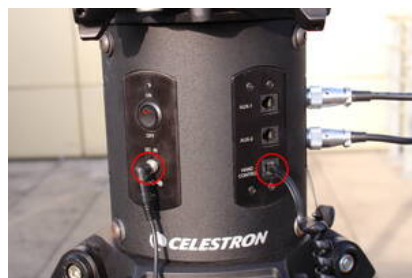
Fig. 12: ports for power supply (left) and terminal (right) at the electronic box
